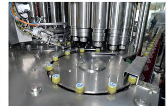
The machine has 3 Section on single frame :Rinsing section with 40 grippers. Filling section with 50 nozzles. Capping section with 12 heads (for plastic caps).
