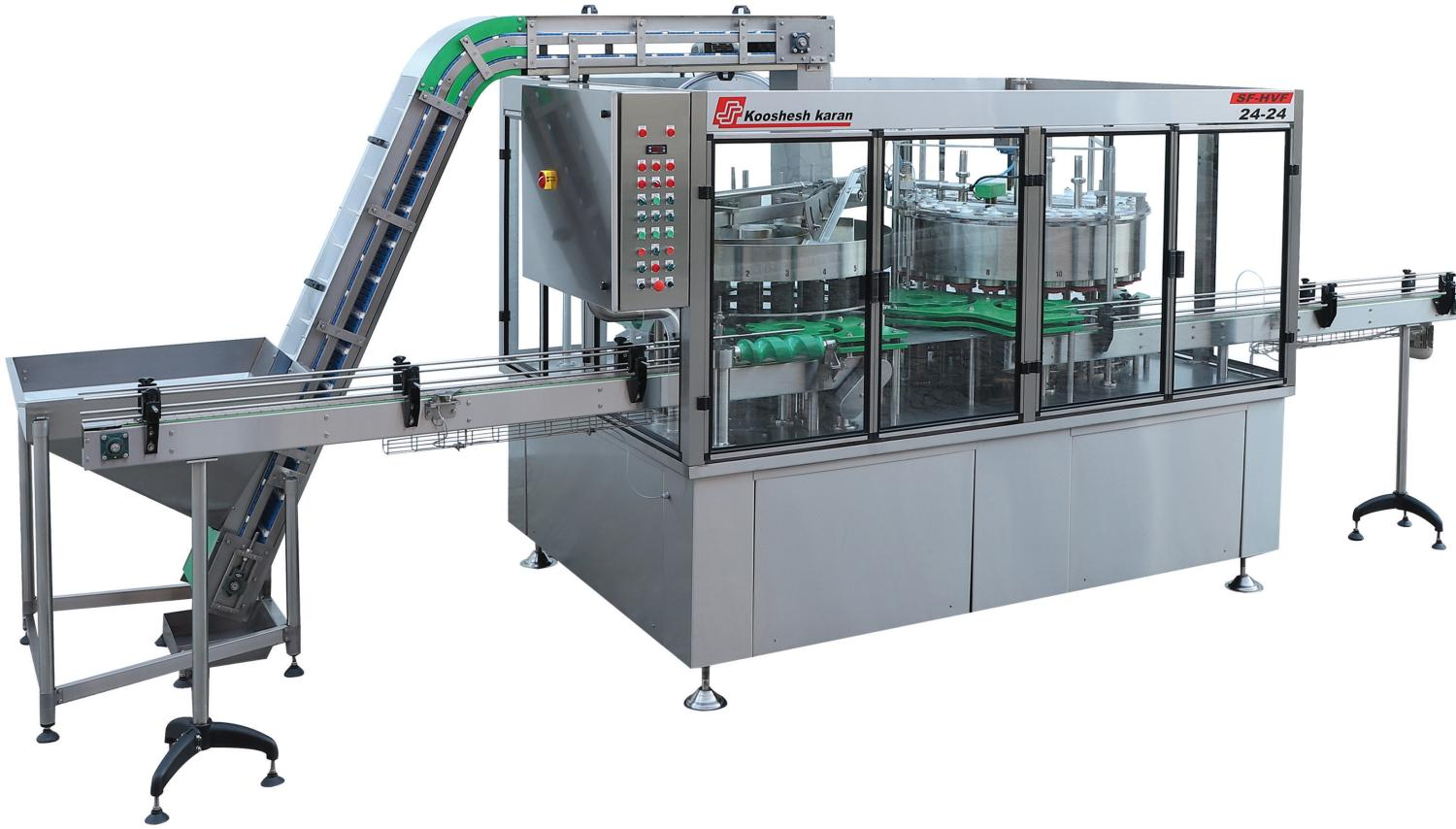
The machine has 2 section ( Solid filler with 24 spots & liquid filler with 12 spots ) on a single frame .
