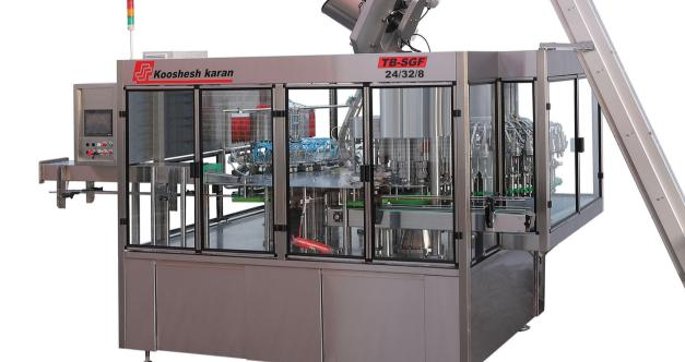
The machine has 3 Section on single frame: Rinsing section with 24 grippers. Filling section with 32 nozzles. Capping section with 8 heads (for plastic caps).
